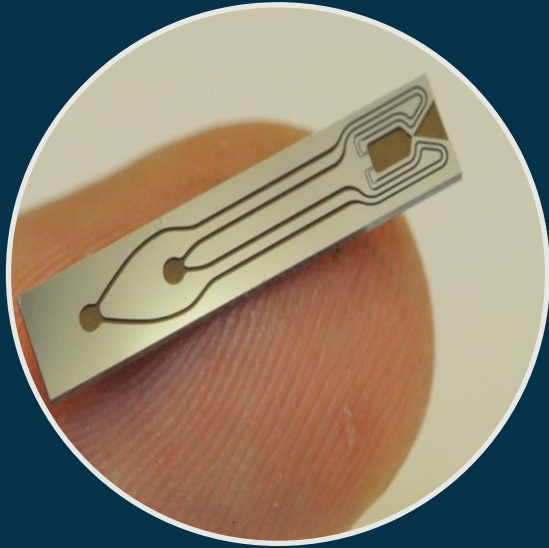
Mini space Thruster that runs on water (URA Thrusters)
